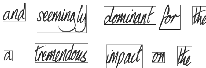
Fig. 2. A section of a page of the database, showing the automatically detected bounding boxes.
