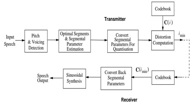
Figure 1. Block diagram of MGPM vocoder structure.
